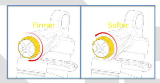
Step 6: High-Speed Compression Adjustment
