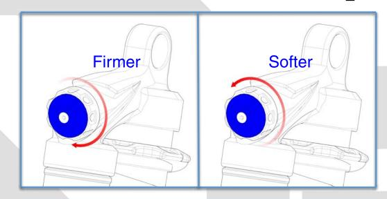
Step 5: Low-Speed Compression Adjustment
